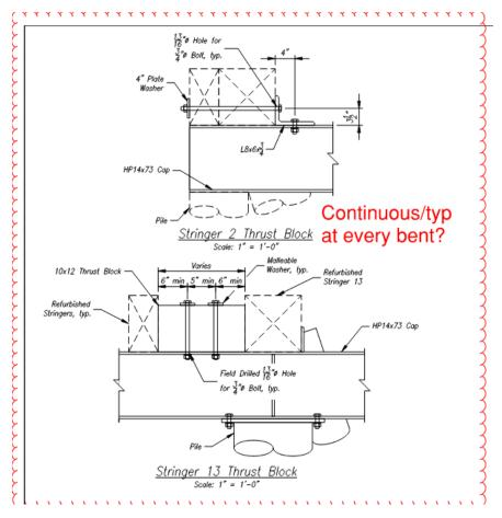
**Response 70.** The L8x6x3/4 and 10x12 Thrust Blocks are typical, bent to bent. The refurbished stringers are continuous. See Section Views on Sheet 80.
